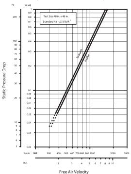
Louver Type SCH7 resistance to airflow varies depending on louver application (air intake or air exhaust). Free area velocities (shown) are higher than the average velocity through the overall louver size. (Test Figure: 5.5-6.5)
